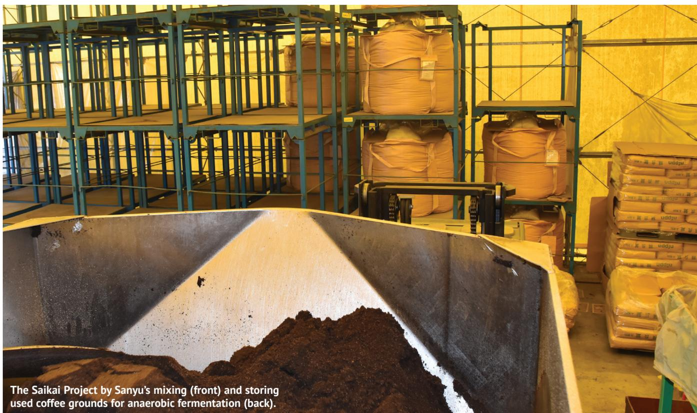
The Saikai Project by Sanyu's mixing (front) and storing used coffee grounds for anaerobic fermentation (back).
